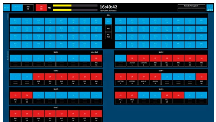
Matrix patching page for allocation of inputs and outputs
